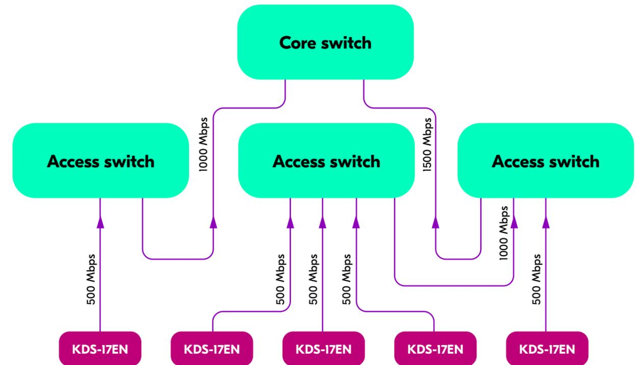
**Downlink:** A port on a switch that connects to an end device (e.g., an AVoIP encoder/decoder, PC, IP camera) or to a lower-level switch (e.g., an access layer switch).
