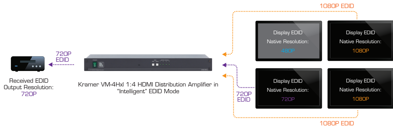
Figure 4b. When the display with the lowest native resolution is disconnected, the distribution amplifier automatically defaults to the next highest resolution supported by all the remaining displays.
