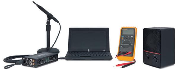
**Advanced Kit** – A senior AV engineer or audio professional typically uses this type of kit for sound system commissioning, which includes gain structure setup and sound power response optimization. Included are one or more calibrated test microphones and a laptop running audio analysis software, together with a multimeter and an acoustical sound source.
