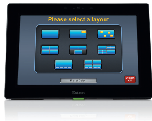
Extron TouchLink® Pro touchpanels can be used to provide a simple user interface to manage selection of videowall display layouts and sources.
