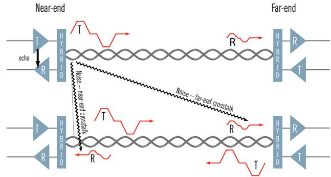
**Figure 2: 1000BASE-T and 10GBASE-T – Bidirectional Transmission**
