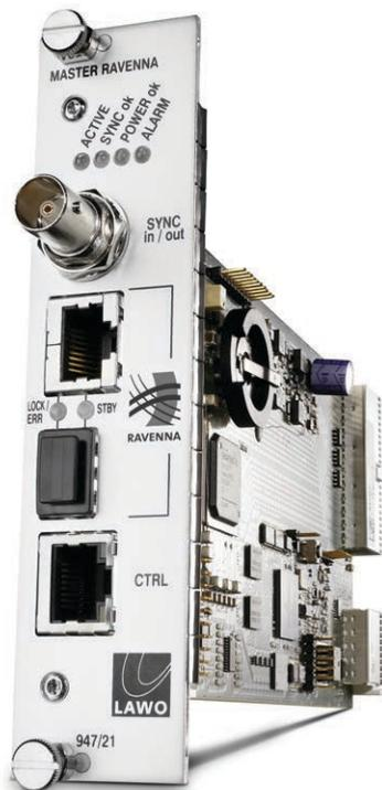
Although they previously used different sync methods, the Axia Livewire XNodes interfaces became RAVENNA compatible with relatively minor changes in field-programmable gate array (FPGA) design and software drivers.
