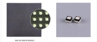
SMD LED has some disadvantages too. SMD dvLED displays are more prone to damage because the LEDs are smaller and more delicate. Also, the SMD LED does not disperse heat as quickly as other types, which can result in higher maintenance costs over the long term.
