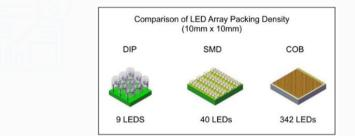
Using COB LED technology can greatly reduce the footprint and energy consumption of the LED array while keeping light output constant. For example, a 500 lumen COB LED array can be many times smaller and consume substantially less energy than a 500 lumen SMD or DIP LED array.
