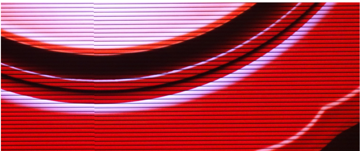
Low refresh rate causes the scan line problem
